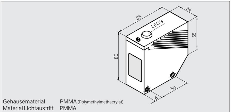
Gehäusematerial PMMA (Polymethylmethacrylat)
