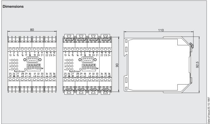
Control Interface with PROFIBUS-FMS Interface, System V
