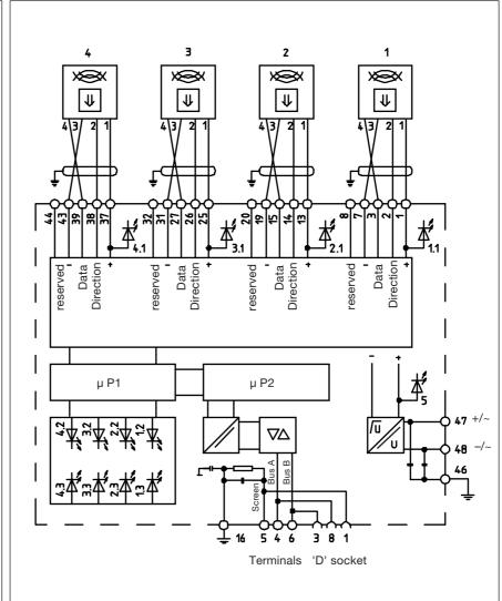
Control Interface with PROFIBUS-FMS Interface, System V
