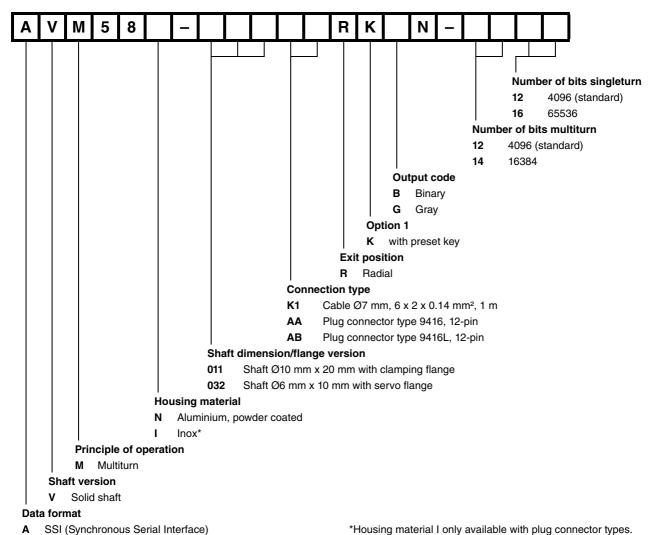
\*Housing material I only available with plug connector types.
