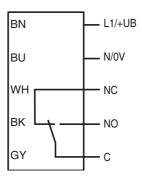
The relay-functions "NC" and "NO" bear on the switching mode "Light-ON".
