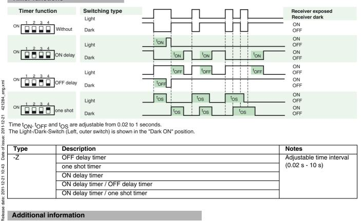
Time  $t_{\mbox{\scriptsize ON}}, t_{\mbox{\scriptsize OFF}}$  and  $t_{\mbox{\scriptsize OS}}$  are adjustable from 0.02 to 1 seconds. The Light-/Dark-Switch (Left, outer switch) is shown in the "Dark ON" position.
