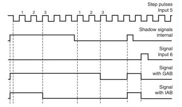
Control of GAB or IAB with incremental pulses on input 5 and by an active signal on Input 6. The setting made for the incremental pulse number is n = 3.
