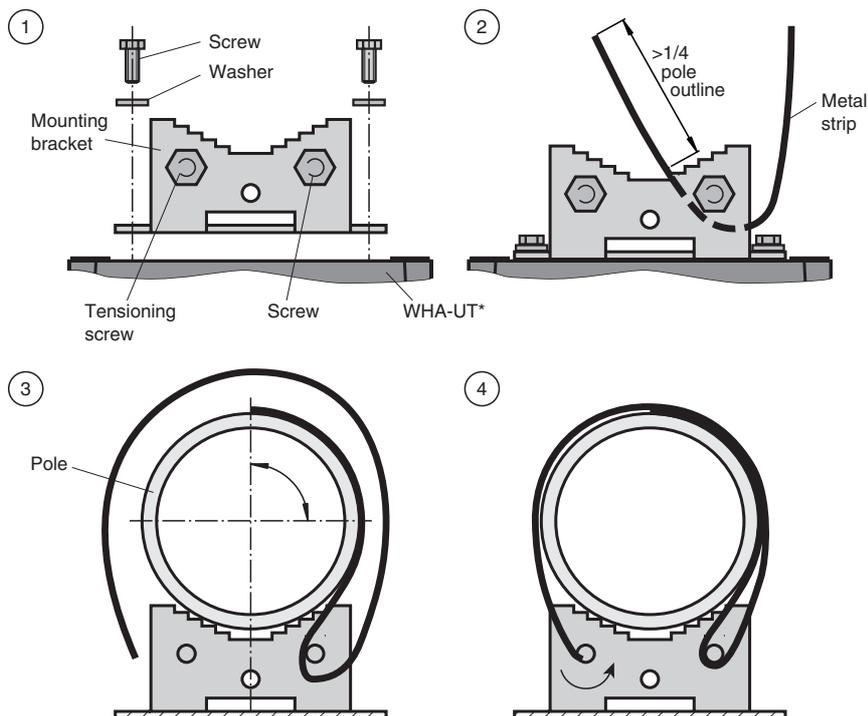
1. Screw the mounting bracket to the backside of the WirelessHART temperature converter WHA-UT-F7B1\*, using the washers and the screws. The orientation is dependant on the orientation of the pole (vertical or horizontal).
