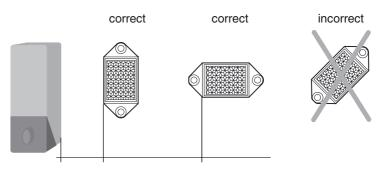
The edge of the sensor must be parallel with the edge of the reflector!
