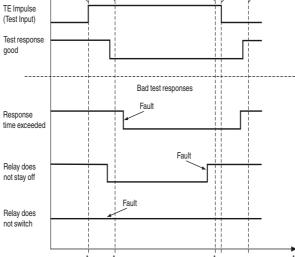
The door controller must query the sensor at times  $t_1$  and  $\hat{t}_2$ .
