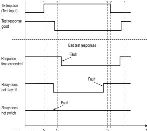
The door controller must query the sensor at times t<sub>1</sub> and t<sub>2</sub>.
