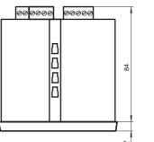
Recommended panel cut-out acc. to DIN 43700: 92 mm + 0.8 mm x 43.5 mm + 0.6 mm (3.6 inches x 1.7 inches)
