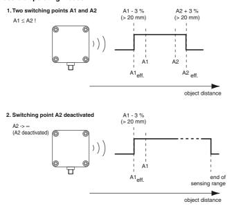
Note: A1 =  $\infty$  is not permitted since A1 must be £ A2. If the switching points are mixed up during programming (teach-in) (A2 < A1), programming will be invalid and the old switching points will be retained. Parameter assignment:
