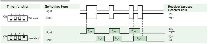
The Light-/Dark-Switch (Left, outer switch) is shown in the "Dark ON" position.
