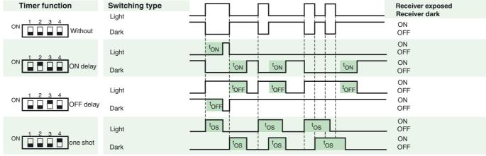
Time  $t_{ON}$ ,  $t_{OFF}$  and  $t_{OS}$  are adjustable from 0.02 to 1 seconds. The Light-/Dark-Switch (Left, outer switch) is shown in the "Dark ON" position.
