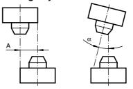
Parallel displacement Angle  $A \le 8 \text{ mm}$
