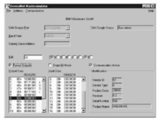
The DeviceNet master simulator is a simple universal machine tool for data exchange with DeviceNet slaves of almost all manufacturers. Input data can be read, output data can be written and diagnostic functions indicated, can be additional without additional input or data files.
