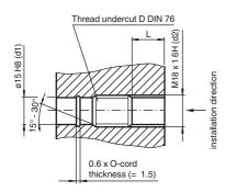
L: recommended installation depth: L  $\ge 0.8 \text{ x d2}$
