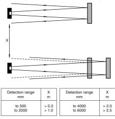
The distance "X" must be observed if two sensors of the same range are installed opposite one another.
