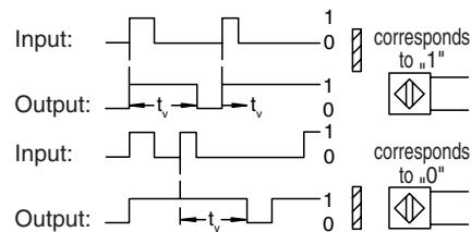
In the case of output diagrams "1" signifies relay energised. The output function can be reversed by changing the mode of operation.
