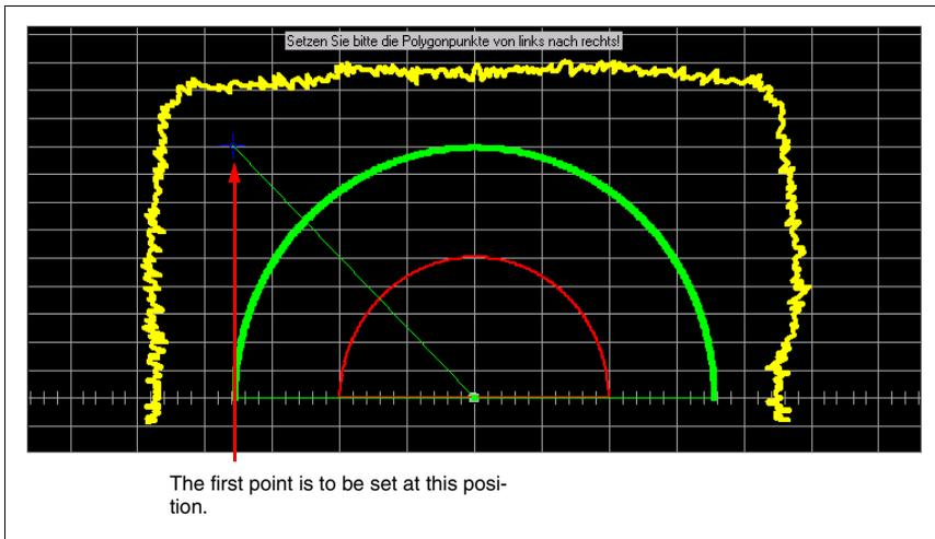
Figure 6.17: Change segment - moving the 1st segment point
