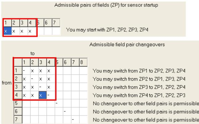
Figure 4.2: Configuring detection field pairs 1 through 4 only
