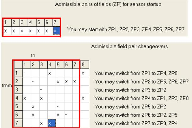
Figure 4.3: Also configuring detection field pairs 5 through 8
