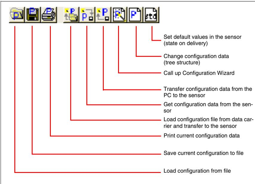
Figure 4.8: Additional buttons in the "Configuration" operating mode
