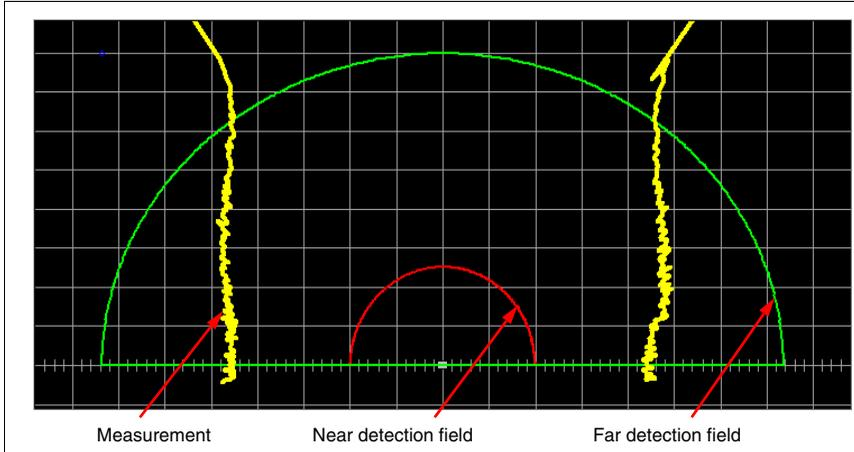
Figure 6.20: Cut detection field - initial situation
