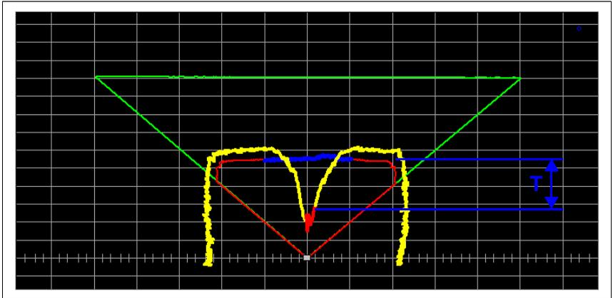
Figure 6.30: Object behind the reference boundary outside of tolerance value T
