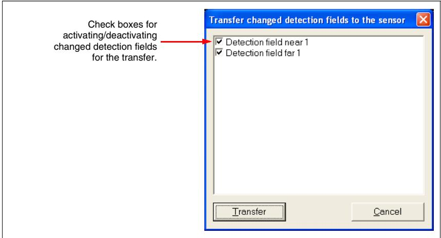
Figure 6.34: Selecting the detection fields to be transferred
