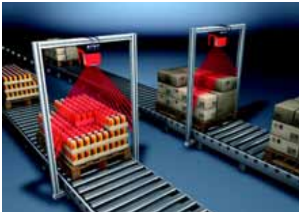
Figure 3.6: Application example - dimension measurement
