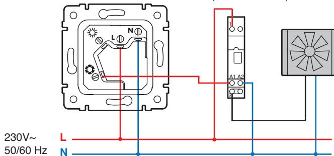
**Attention:** Distribution voltage to be connected cophasally to thermo regulator and remote control. Installation and assembly may only be effected by an expert!
