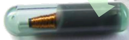
biocompatible glass transponder for underskin injection in livestock
