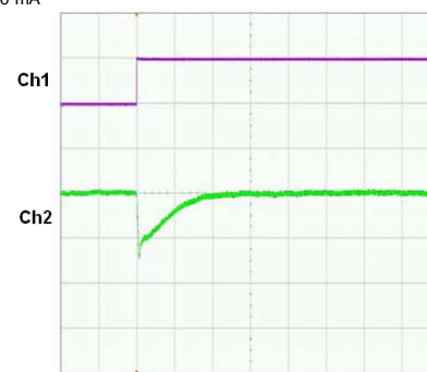
Ch1 – I_{OUT} , Ch2 – V_{OUT} 50 mV/div, Time – 50 \mu\text{s} /div
