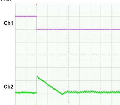
Ch1 – I_{OUT} , Ch2 – V_{OUT} 50 mV/div, Time – 200 \mu\text{s} /div
