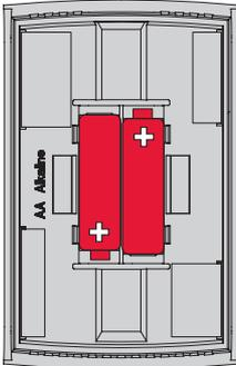
Install 2 AA alkaline batteries
