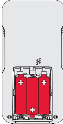
Install 3 AA alkaline batteries
