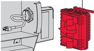
**3** Clean the back panel inside the wiring compartment where the relay will be installed. Peel the adhesive backing off the relay and stick the relay on the back panel.
