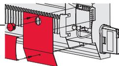
**6** Put the heater cover back. (If a built-in thermostat was removed, install one of the supplied plugs to cover the hole on the existing cover.) Apply power to the heater. Do not install the antenna cover yet.
