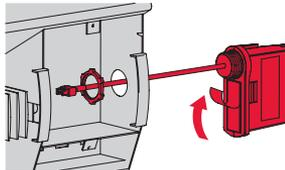
**2** Remove the locknut from the antenna and peel off the adhesive backing. Feed the antenna cable through the knockout and install the antenna vertically as shown. Put the locknut on and tighten.
