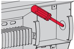
**1** Remove the knockout on the side of the heater.
