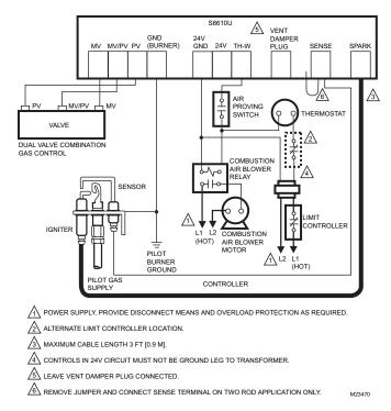
Fig. 10. VR8245M/VR8345M,H wiring connections in intermittent ignition system.
