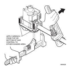
Fig. 6. Proper use of wrench on gas control.
