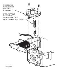
Fig. 5. 396021, 396025 two stage conversion kit installation.
