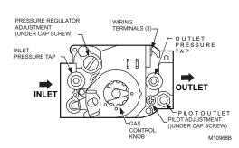
Fig. 3. Top view of gas control.
