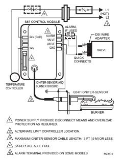
Fig. 12. VR8245M/VR8345M,H wiring connections in direct spark ignition system (single rod application).
