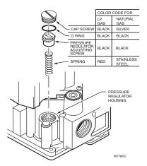
Fig. 4. 393691, 394588 Coversion kit installation in regulator
