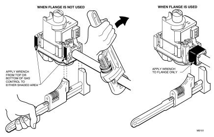
NOTE: When replacing a gas control, cut off old compression fitting and replace with the new compression fitting provided on the gas control. Never use the old compression fitting because it may not provide a gas-tight seal.
