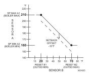
Setting up the reset on the Honeywell T775R is a breeze. Just enter the minimum and maximum boiler temperatures and the corresponding minimum and maximum outdoor temperatures — and that's it. Your reset curve is complete and the
