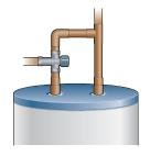
AM-1 mixing valve installation.
