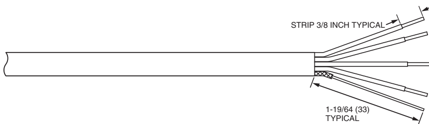
Fig. 5. C330S Signal Processor End Cable Preparation.
