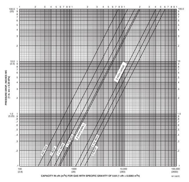
Fig. 4. Flow curves for V5097 valves.
