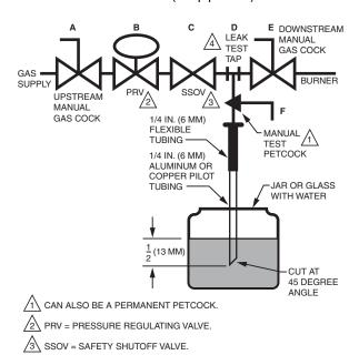
Fig. 5. Valve leak test.
