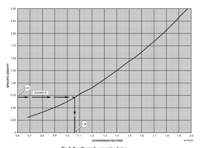
Fig. 3. Specific gravity conversion factors.
