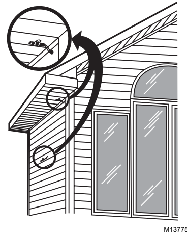
Fig. 7. Outdoor temperature sensor installation.
