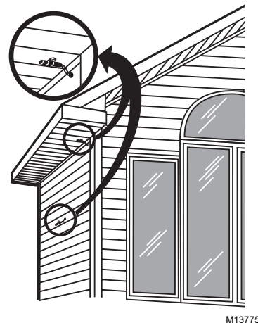
Fig. 7. Outdoor temperature sensor installation.
