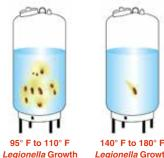
Honeywell mixing valves are designed to prevent the growth of bacteria by allowing you to set your water heater at 140° F.
