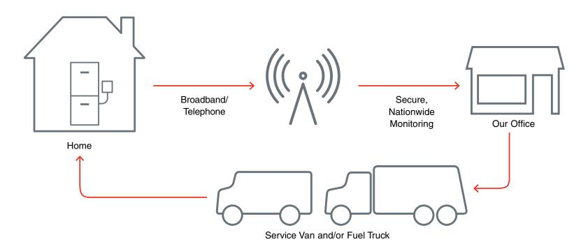
EnviraLINK<sup>®</sup> uses the EnviraCOM<sup>™</sup> protocol built into your heating and cooling equipment to diagnose your oil and maintenance needs and then reports to us anytime, day or night.
