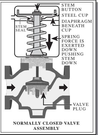
Normally open and normally closed are terms that refer to the position of an actuator and valve or actuator and damper assembly when the power is removed. Coils are prevented from freezing in an airhandler if the coil has full flow through it during the off cycle. Similarly a reheat coil on a variable air volume box does not require freeze prevention and the actuator should be closed if there is no airflow to prevent tripping plenum heat detectors.
