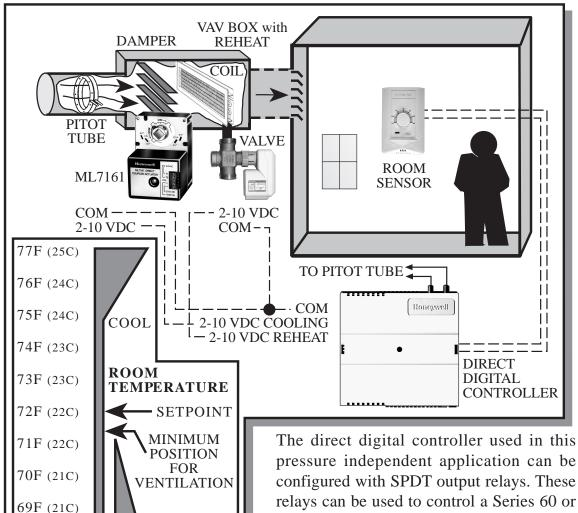
Series 70 devices use 0 to 10 volts dc (Vdc), 2 to 10 Vdc or 4 to 20 milliamp (mA) control circuits. These control circuit voltages are very prevalent today, making replacement of other company's actuators with Honeywell devices economically feasible. Series 70 is intrinsically modulating with actuator feedback either built into the signal voltage or from a feedback potentiometer. Both actuators in this illustration are supplied with 24 volts AC.
