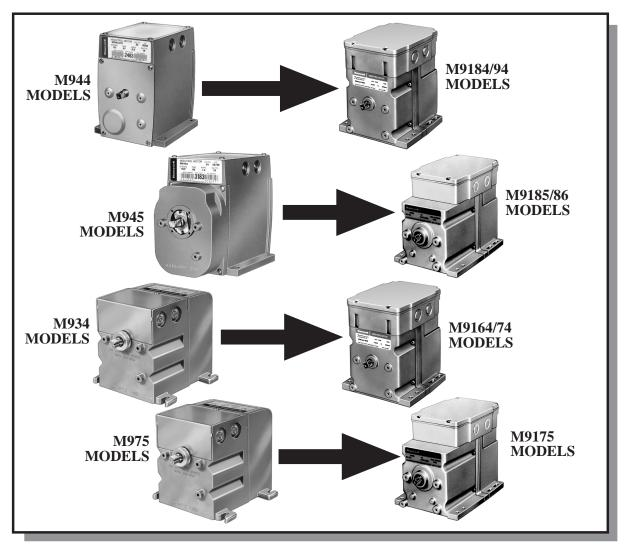
While Honeywell provides a complete line of direct coupled valve actuators there are many retrofit applications where it is preferrable to replace a modutrol motor with a similar motor. This could be due to high torque requirements or inability of removing insulation from the linkage. The Mod IV line of motors is available to replace virtually all previous Honeywell actuators and can be adapted to the existing linkage if necessary. A newer Q5001 valve linkage is also available.
