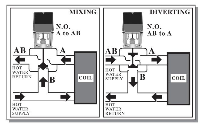
Three-way valves are primarily used for water applications and infrequently to switch compressed air. It is typically open to one port or the other. There are smaller three-way valves which sequence ports and can be closed or open to both ports simultaneously. Most of the larger valves though, are of the type illustrated here and would be labelled "Normally Open A to AB", or "Normally Open AB to B."
