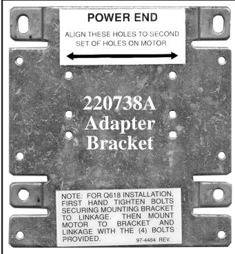
The shaft heigth on the Honeywell Mod IV motors is 3/4 inches (2 cm) lower than that of the previous line of motors the Mod III. When replacing Mod III actuators in valve applications without replacing the Q618 linkage, an adapter plate is required. This adapter, which raises the heigth of the shaft 3/4 inches (2 cm) has been included in the box with some motors. This plate is installed on the valve linkage first. The Mod IV actuator is then bolted to the plate.
