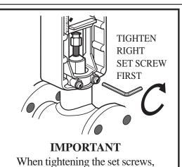
Attach the actuator to the valve collar and tighten the set screws with a 5/32 inch (4 mm) hex wrench.
