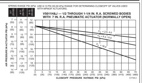
ACTUATORS USED. THREE-WAY VALVES WILL FREQUENTLY BE LISTED WITH TWO CLOSE-OFF RATINGS, ONE FOR EACH SEAT.
