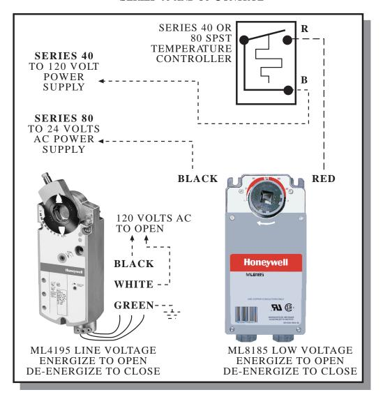
Series 40 and 80 are identical except for the voltage of the control circuit. Series 40 is line, typically 120 volts AC, while Series 80 is low, typically 24 volts AC. A controller with SPST switching, similar to a light switch, is used. The actuator is energized and repositioned fully to its other position. When the ambient temperature, or control point, is attained the controller switch is opened, the actuator is de-energized and it is spring returned to its normal position.
