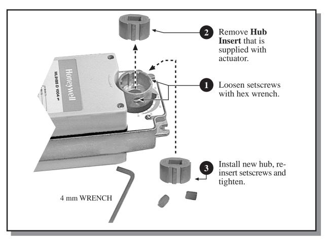
The hub insert is replaceable on the 50 lb-in (6 N-m) line of actuators. They are typically supplied with a 1/2 inch (13 mm) insert. There are three replacement hub inserts available. These are primarily for use with damper shafts and will probably not be used with ball valves since most ball valves linkages from Honeywell are either
