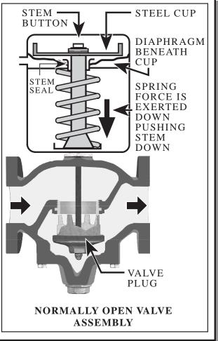
These are the same two actuators as on the previous page. The valve however is stemdown-to-open which reverses the normal position of the two assemblies.
