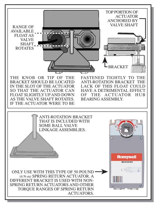
There are several ball valve linkages and each is designed to be used only with certain actuators. One or more anti-rotation brackets are included with the ball valve. These are designed to anchor the back of the actuator so it does not spin. It must
