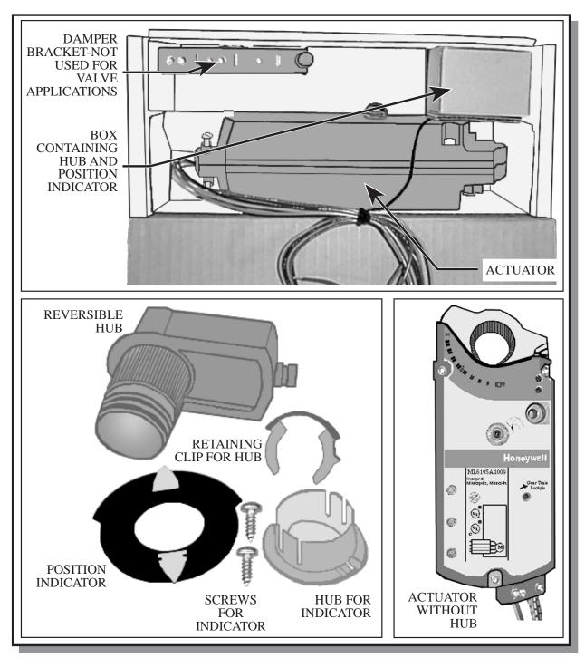
This is the components of a 142 lb-in (17 Nm) actuator. Other torque ranges will be slightly different so refer to the literature for instructions. This actuator is supplied in a box with all of the components necessary for a damper installation. The bracket and
