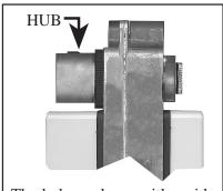
The hub can be on either side of the actuator though it is best to have it on the side away from the valve if the actuator is set for a normally open valve. Its position does not affect the direction of spring return or the control output.
