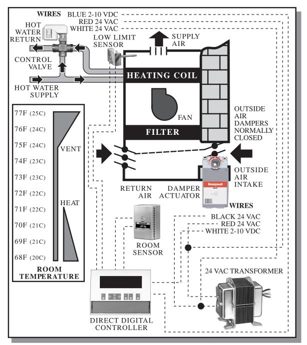
If the room becomes warm and the heating valve closesd the supply air temperature can drop too low and cause cold drafts in the room. A supply air low limit prevents this by opening the heating valve if the supply temperature decreases below 55 or 60 Deg. F (13 or 16 C). Once the supply air temperature rises above the low limit
