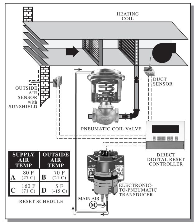
Transducers are used to take an electronic signal from a controller and convert it to a pneumatic signal to modulate a valve or damper actuator. This is frequently on on mixed air dampers since multiple large damper motors can be connected to one
