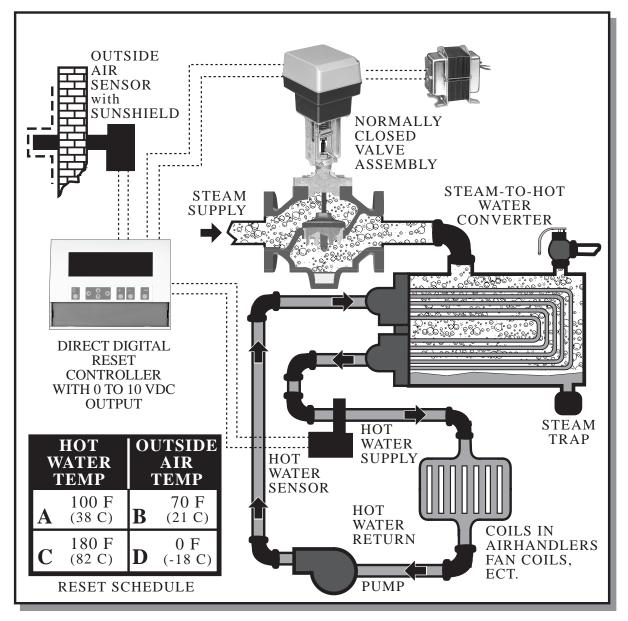
Most modern buildings are heated with hot water boilers. Facilities constructed prior to 1940 were probably heated with steam. Additions to these buildings are typically hot water heat due to its controllability, safety and maintenenace benefits. The use of a steam-to-hot-water converter permits retaining the steam boiler while heating new areas of the building with hot water. Other facilities such as hospitals and industrial facilities often require the
