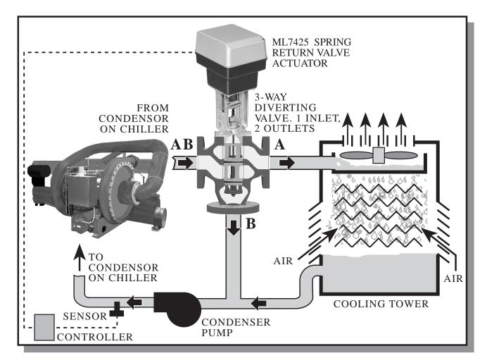
Chillers are used to generate chilled water to cool a building. While some of these are paired with air cooled condensors most of the larger units are connected to cooling towers. Cooling towers are used to dissipate the heat taken from inside of the building to the outdoors. A valve is generally required to control the temperature of the condensor water being returned to the chiller.
