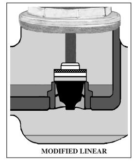
In the Honeywell Valve Selection Guide 63-8038 valves are listed with the options available for each. Some of them are listed with a plug referred to as a modified linear. This is a plug that is primarily linear for approximately 90% of the stem lift. 10% is curved similar to an equal percentage plug to improve modulation at low flow rates. Most valves using this plug are metal-to-metal seating and are primarily for steam modulation.
