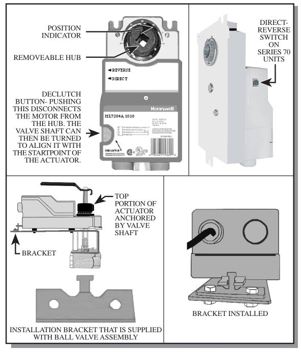
The non-spring return actuators are installed on the flat back side only. Direct-reverse adjustments are done on series 70 units with a switch on the side. The mounting hub is reversible but will portrude substantially when installed from the back. Hub inserts are available
