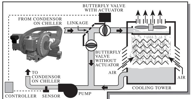
Few mixing or diverting three-way valves are available commercially in larger pipe sizes. To provide two-position or modulation control two butterfly valves can be used. In this illustration there is only one actuator and the second valve is controlled with a linkage connected to the first. Two actuators without connecting linkage can also be used if the actuators can be made to modulate in unison.
