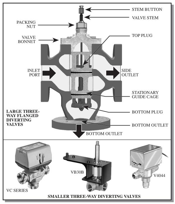
Diverting valves are used to take a single input flow of water and divert it to either of two ports. Some of the smaller valves can be piped backward to become a mixing valve. The larger valve illustrated above though cannot be piped backwards without incurring damage
