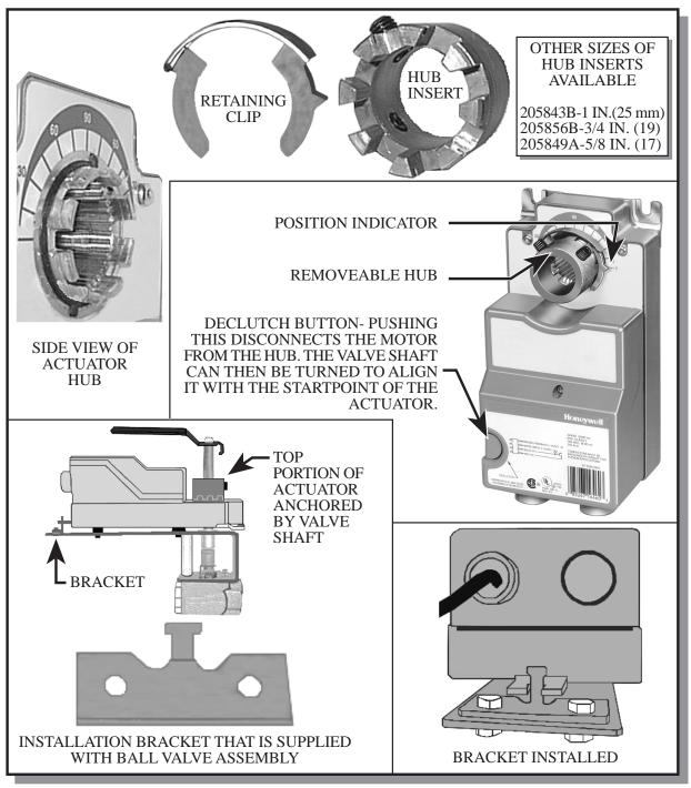
The 300 lb-in (34 N-m) non-spring return actuators are installed on the flat back side only. Direct-reverse adjustments are done on series 70 units with a switch on the side. Hub inserts are available for various shaft sizes but only the 1/2 or 1 inch inch (13 or
