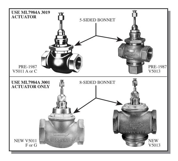
Honeywell's commercial globe valves were modified in 1987. In addition to changes in the disc and seat configurations the shape of the bonnet was altered. This affected the use of the ML7984 actuator. The amount of close-off changes from the pre-1987 valves to the newer ones when a ML7984 is used. This is caused by the change in effective stem lift when
