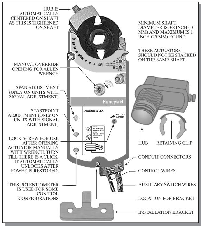
This is a 142 lb (16 N-m) actuator with a self-centering hub. High torque spring return actuators are among the most widely used type in heating, ventilating and air conditioning applications. Spring return is
