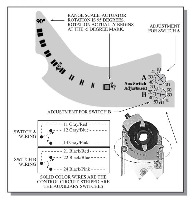
This line of actuators is available with and without auxiliary switches. If there are no switches there will be no dials inside the scaleplate. It is recommended to set the **A** switch to a lower value, such as between 0 and 45 degrees rotation and the **B** switch to a higher value, such as 45 to 90 degrees. The switch differential is 5 degrees for each switch.
