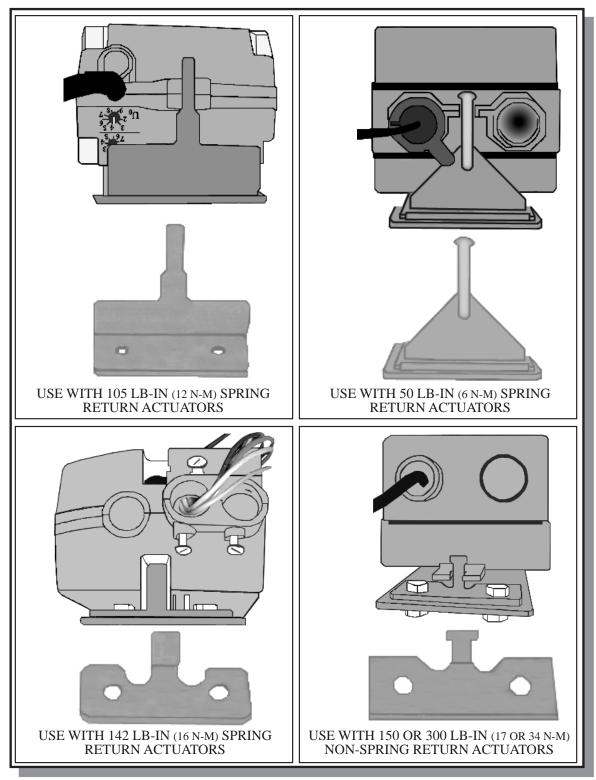
There are many ball valve and actuator combinations available. There are four antirotation brackets available for the medium and large direct coupled actuators. Only one of them is used for any single valve. Bolts are included in the package.
