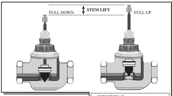
Valves are available as unitary or assembled units. The difference is that a unitary valve is designed to be used with a specific actuator. Unitary valves are typically smaller valves. An assembled unit consists of one of Honeywell's threaded or flanged valves and one of a wide selection of actuators. The actuator can be electric or pneumatic, spring return or non-spring return or one of any of the available close-off ratings.
