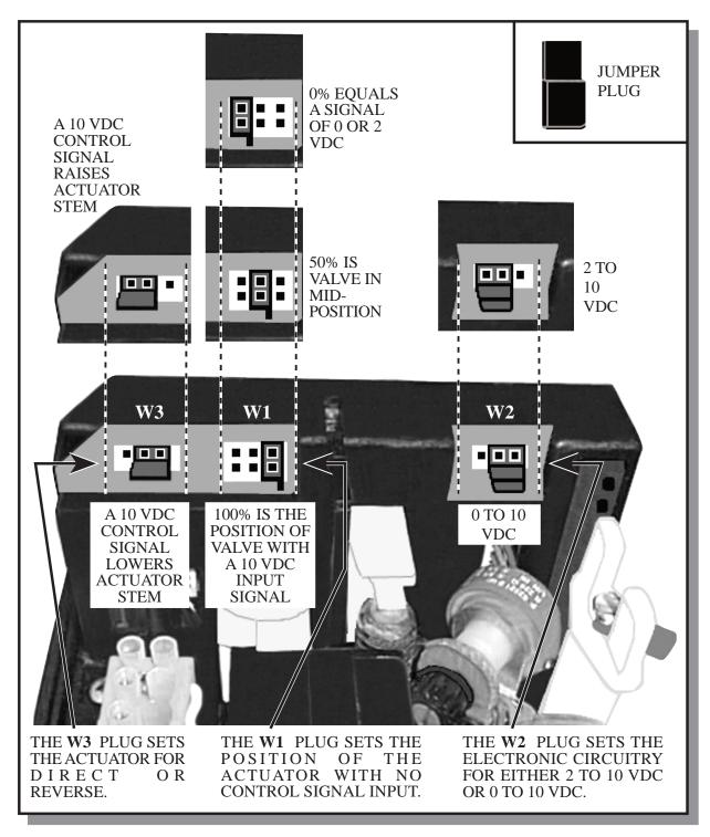
There are 3 jumper plugs on the circuit board of the ML7425 which are used to make 3 separate adjustments. Each
