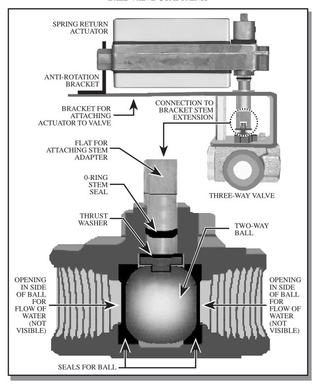
The bracket for ball valves is fastened to the top of the valve with bolts that are threaded into the body. The stem extension is fastened to the valve stem without any setscrews or bolts. Brackets are available for use with the various direct coupled actuators that Honeywell produces.
