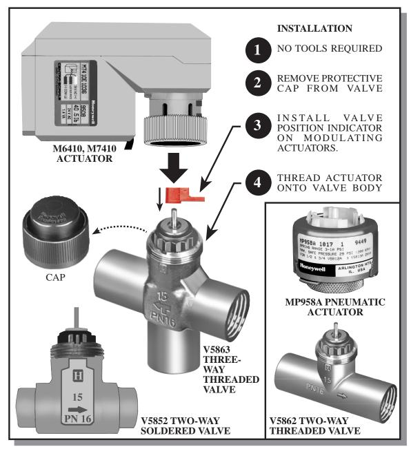
V5852/53 and V5862/63 are two and three-way valves available 1/2 (1.25 cm) and 3/4 inch (1.9 cm) threaded and soldered with a Cv up to 4.9. The three-way valves are mixing. They are widely used on variable air volume box applications since the noise level is very low. A valve assembly that is audible during the opening or closing cycle can be
