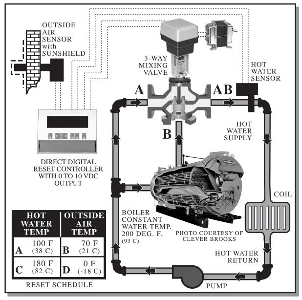
The water used to heat a building is typically supplied from either a boiler or a steam-to-hot water converter. The building illustrated here is heated from a boiler. The temperature of the water should be varied inversely with the outdoor air temperature. This is referred to as hot water reset and it reduces overheating during moderate weather. The required temperatures are listed in the reset schedule.
