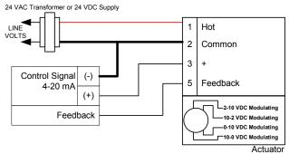
Note: Set signal DIP Switch under Access Cover to Current
