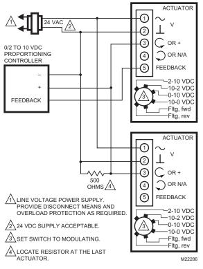
Fig. 44. 4-20 mA control of multiple actuators.
