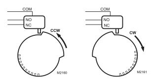
Fig. 52. Fast-acting two position actuator switch package.
