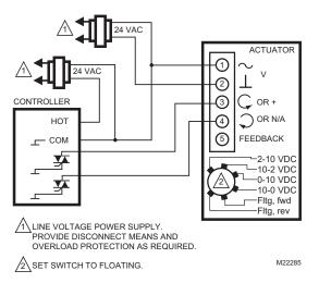
Fig. 22. Low-side triac floating S05, S10, S20 Series (MS81XX, MS41XX, MS75XX) with separate transformers.
