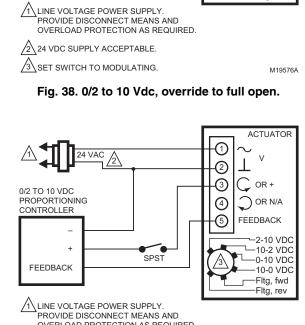
Fig. 39. 0/2 to 10 Vdc override to full closed.
