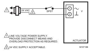
Fig. 6. MS81XX, two-position actuation.
