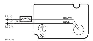
Fig. 14. ML4X02F, ML4115A-D, ML4X09F (230 Vac).
