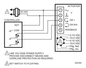
Fig. 21. Low-side triac floating S03, S05, S10, S20 Series (MS81XX, MS41XX, MS75XX).
