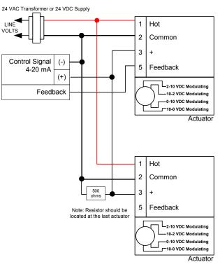
Fig. 33. Single transformer, wired in unison.
