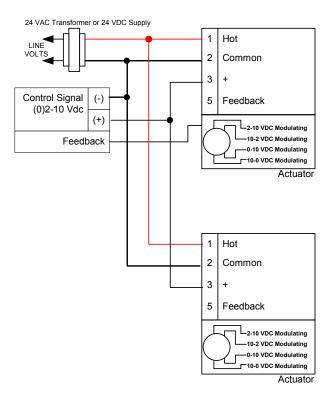
Fig. 30. Single transformer wired in unison.
