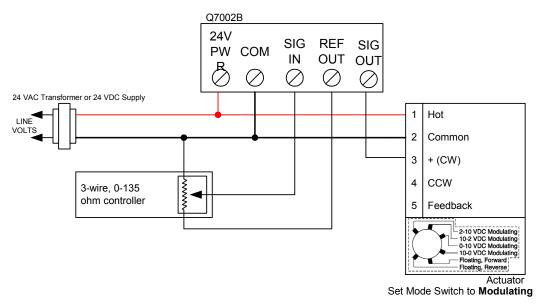
Fig. 47. 135 ohm control of S03, S05, S10, S20 Series (MS75XX).
