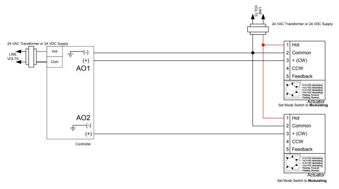
Fig. 2. Corrected wiring without ground loop.
