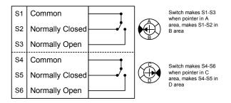
Fig. 49. SW2-US Auxiliary Switch wiring.
