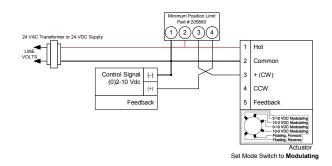
Fig. 45. 0/2 to 10 Vdc control.
