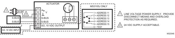
Fig. 40. Wiring for Sylk BUS, MS3103, 05 series.
