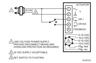
Fig. 19. Standard floating S03, S05, S10, S20 Series (MS81XX, MS41XX, MS75XX).
