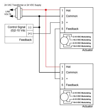
Fig. 31. Single transformer, master drone.
