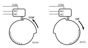
Fig. 50. ML6161/74 switch package.
