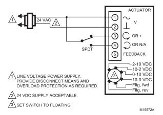
Fig. 10. MS75XX using spdt, 3 wires from the controller.
