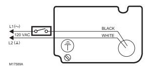
Fig. 13. ML4X02F, ML4115A-D, ML4X09F (120 Vac).
