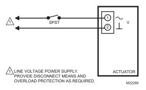
Fig. 7. MS41xx, two-position actuation.
