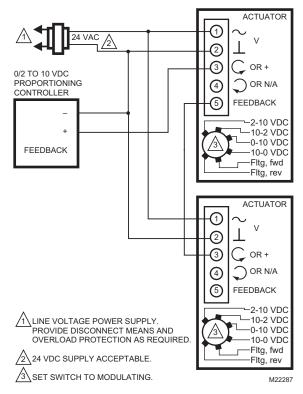
Fig. 43. (0) 2-10 Vdc control as master drone.
