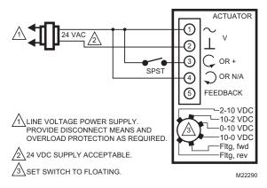
Fig. 8. MS75XX using spst, 3 wires from the controller.
