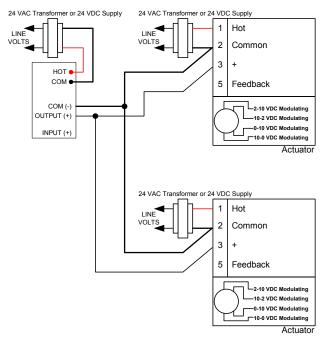
Fig. 32. Separate transformers, wired in unison.
