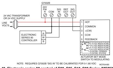
Fig. 48. Electronic series 90 control of S03, S05, S10, S20 Series (MS75XX).
