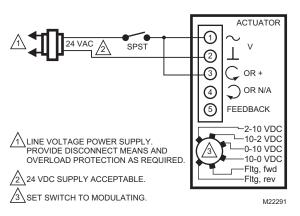
Fig. 9. MS75XX using SPST, two controller wires.
