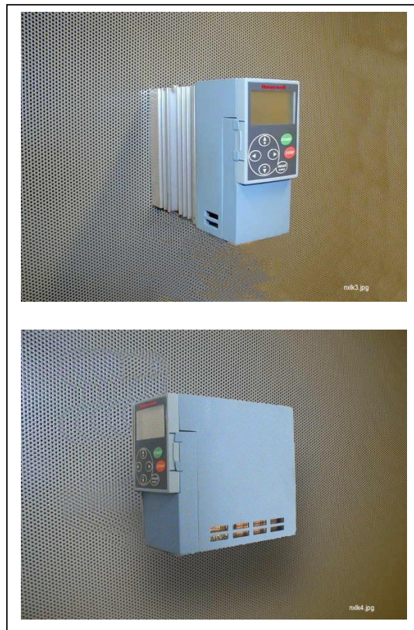
Figure 5-1. The two possible mounting positions of NXL (MF2 and MF3)
