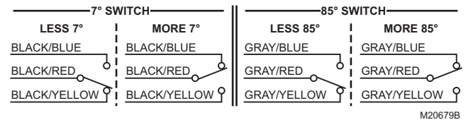
Fig. 12. SPDT auxiliary switch operation.
