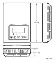
Fig. 11. Thermostat dimensions in inches (mm)
