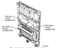
Fig. 3. Re-install terminal blocks
