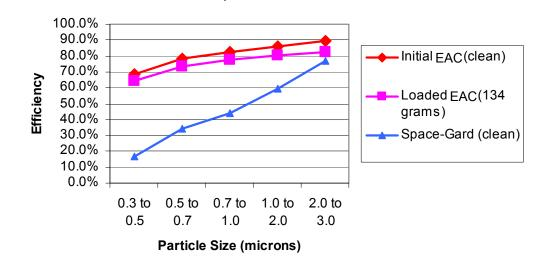
Testing was conducted using test dust defined in ASHRAE Standard 52.1. This dust contains carbon, which is electrically conductive, which tends to impact the efficiency more than a non-conductive dust.
