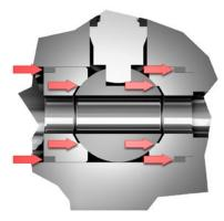
The forces required to maintain the tightness are stressing all components - even the ball and seats. The operating torque is thus very high.
