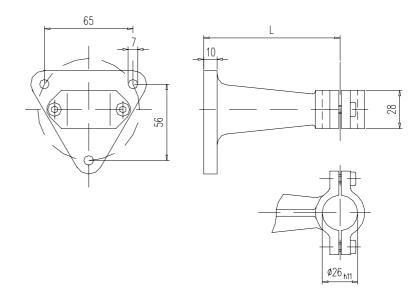
**Design A** for mounting to 2" NB pipes, wall or racks
