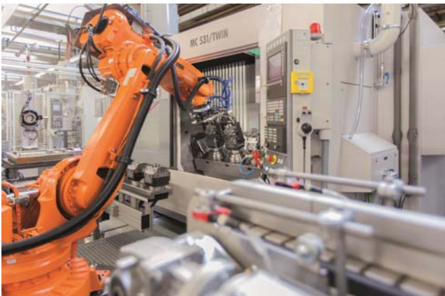
Double-spindle machine – The new clamping concept allows twice the amount of production per manufacturing cycle
