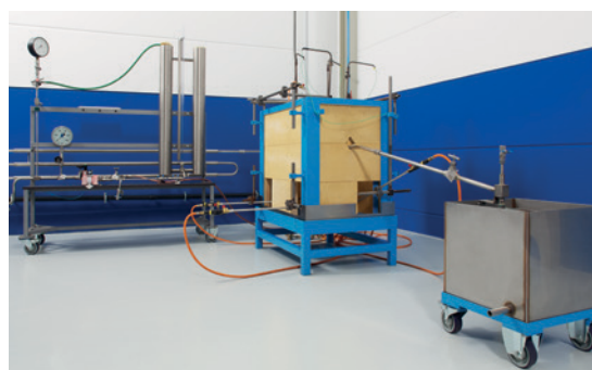
Fire Safe Test Bench For testing valves with sizes up to 2"
