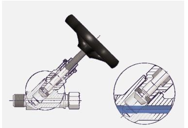
**Y-Pattern Needle Valves Type S371:** Minimize flow velocities and, therefore, decrease the erosive forces which shorten the life of the valve tip and seat. The valve can also be rodded if plugged.
