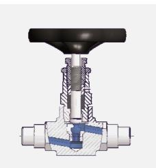
**Straight Pattern Needle Type Globe Valves:** The stem is vertical to the flow direction. The flow must therefore be deflected by about 90° twice. This results in high pressure losses.
