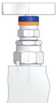
Colour Coded Option FKM O-Ring Stem Seal with PCTFE Soft Tip
