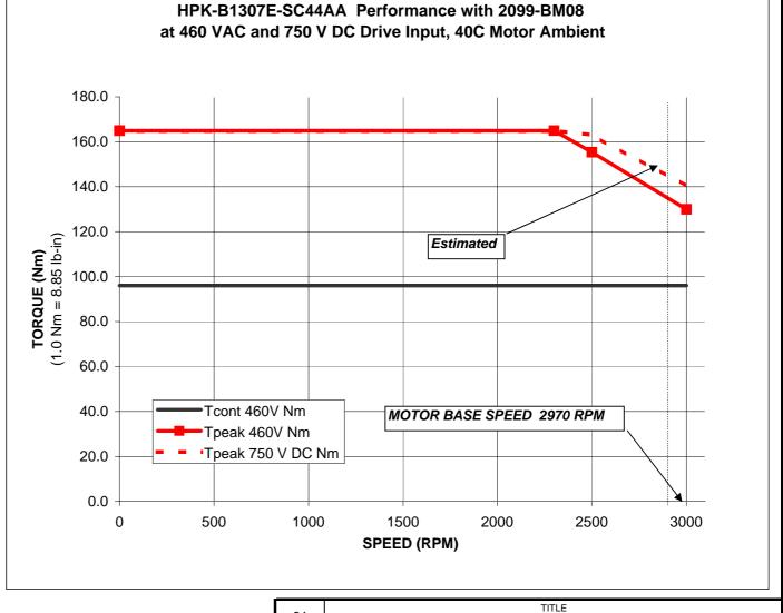
Note: Nm torque values shown are converted from tested lb-in data.
