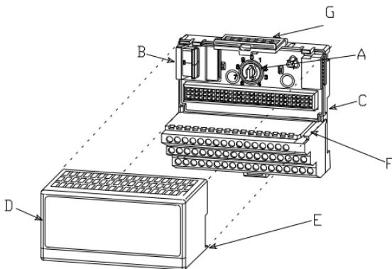
2. Make certain the side connector (B) is pushed all the way to the left. **You cannot install the module unless the connector is fully extended.**
