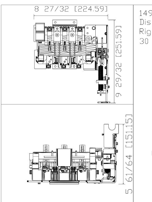
1494C-D\*3\* Disconnect Switch Kits, Right-Hand Mechanism, 30 Amp
