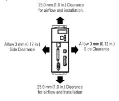
Allow additional space for side mount or rear mount AC line filters. See the table and Kinetix 300 AC Line Filter Installation Instructions, publication 2097-IN003.
